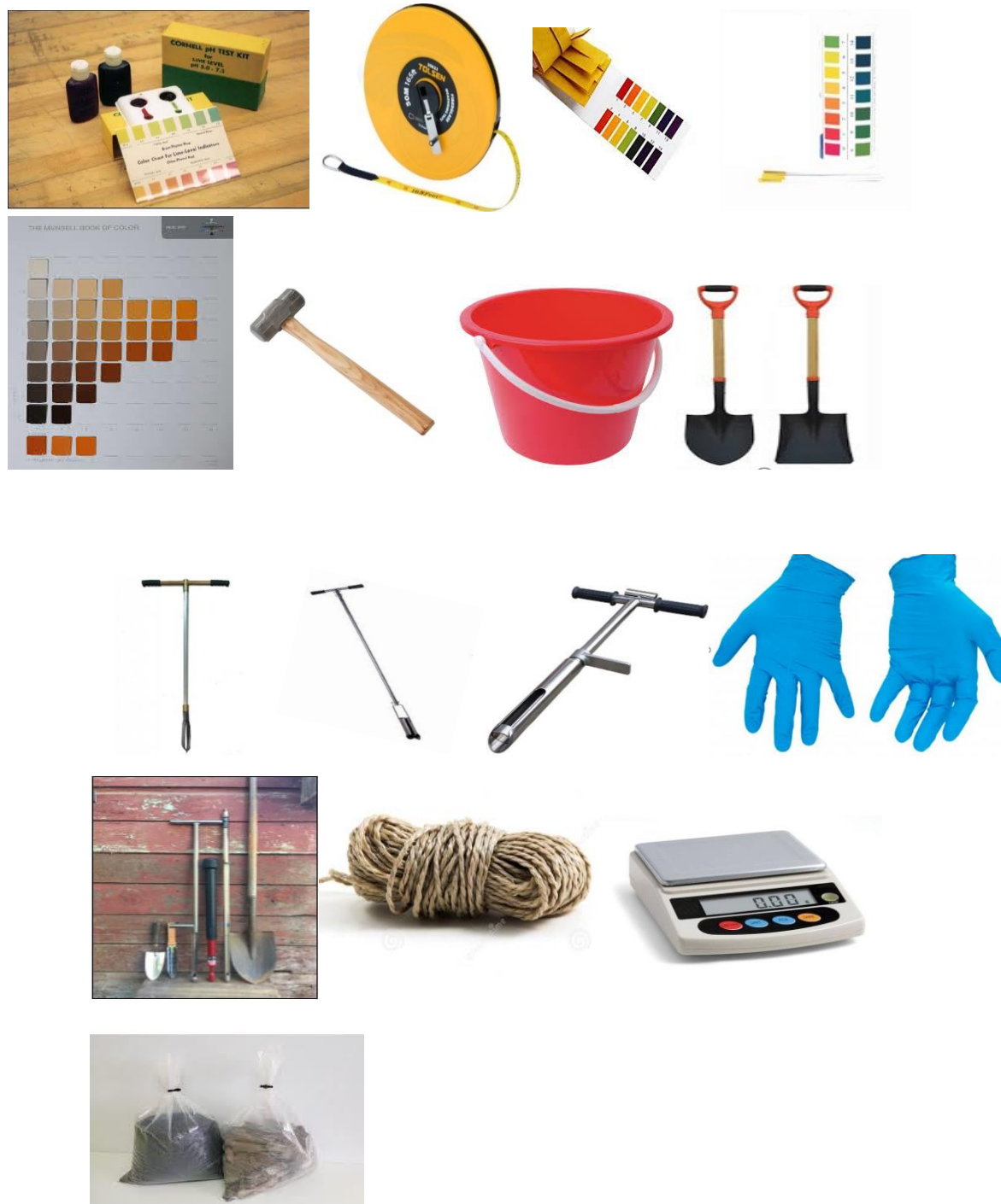
Figure: 1:2 Tools and equipment needed for soil sampling and testing
